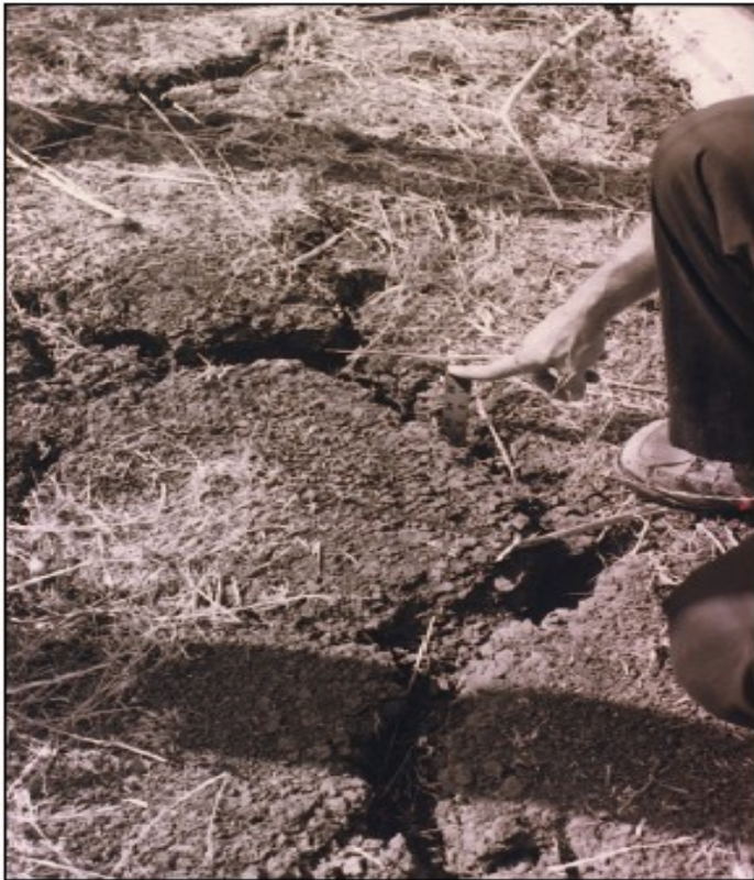
Photo 2: This crack is at least 32 inches deep. The yardstick was easily inserted to this depth; narrower, less straight cracks may extend much deeper.
