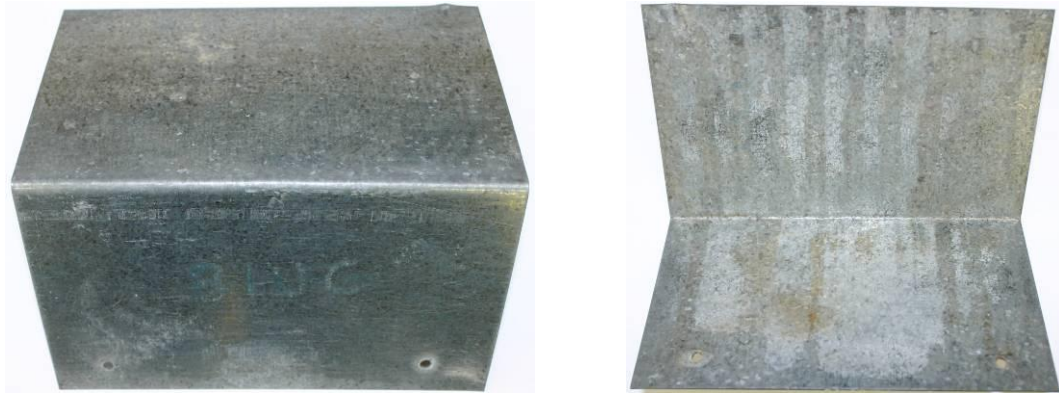
Figure 11: Surface morphology of hot dip galvanised steel flashing attached to untreated timber exposed at Judgeford site for one year
