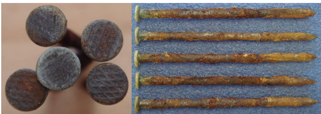
Figure 54: Hot dip galvanised steel nails embedded into H4 ACQ treated timbers exposed at Judgeford site for three years. The formation of iron-rich red rust on the top surface of the head is not as severe as on the shaft
