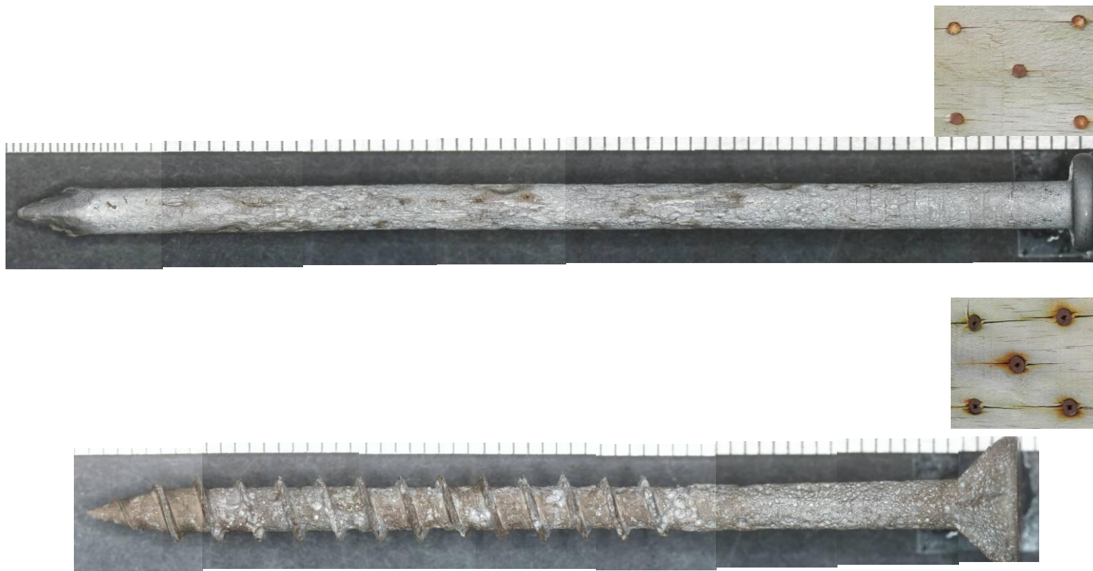
Figure 55: Cleaned zinc-coated fasteners retrieved from H4 ACQ treated timbers exposed at Oteranga Bay for three years. The zinc coating on the head was consumed and then iron-rich rust was formed. However, it must be noted that corrosion on the body section was still more severe than on the head
