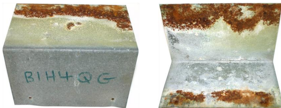
Figure 9: Surface morphology of hot dip galvanised steel flashing attached to timber exposed at Judgeford site for one year – the timber was treated with H4 ACQ
